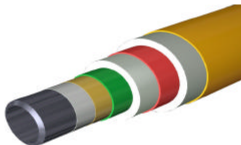
Figure 1. Thermal Insulation System for Single Flowline
