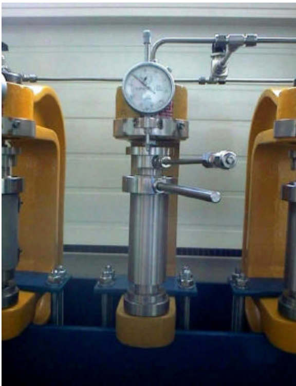
Figure 4. Photography of the Tri-Axial Test Method Set-Up
